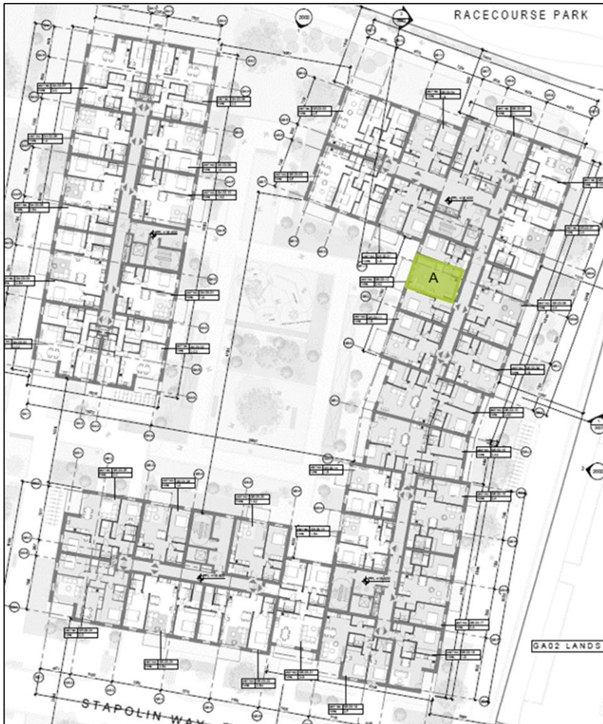
Figure 15.25: Blocks G4/G5 Third Floor Level – Average Daylight Factor Assessed Rooms
