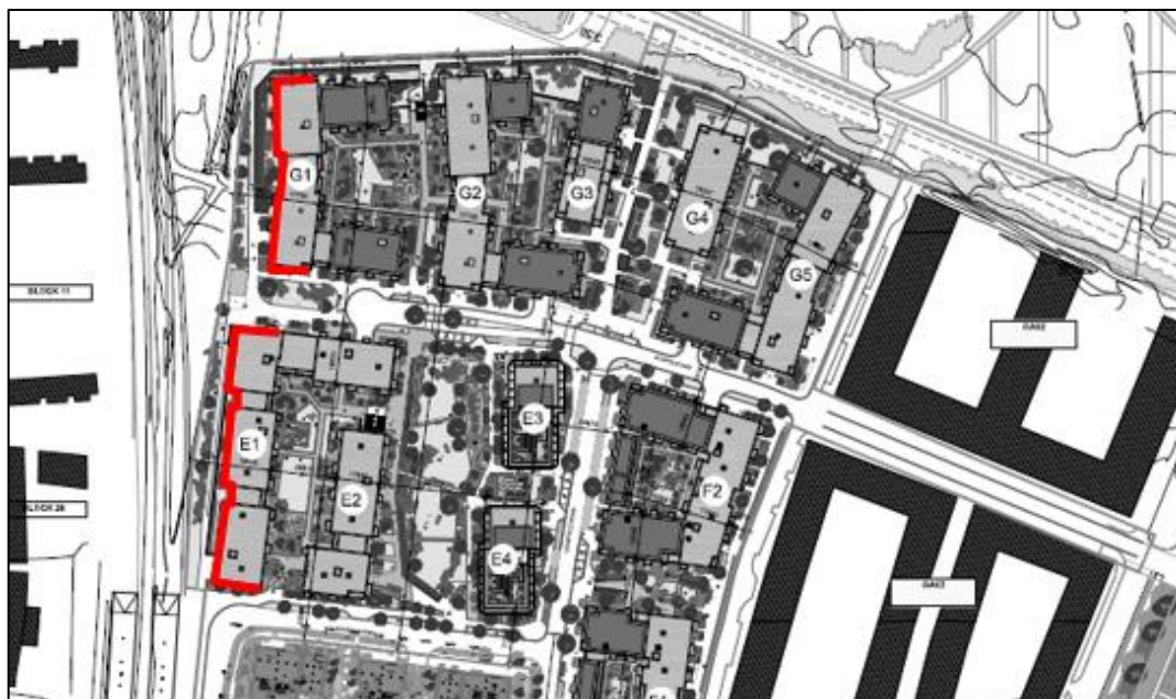
Figure 12.7: ProPg Stage 2 – Façade Sound Insulation Requirement
