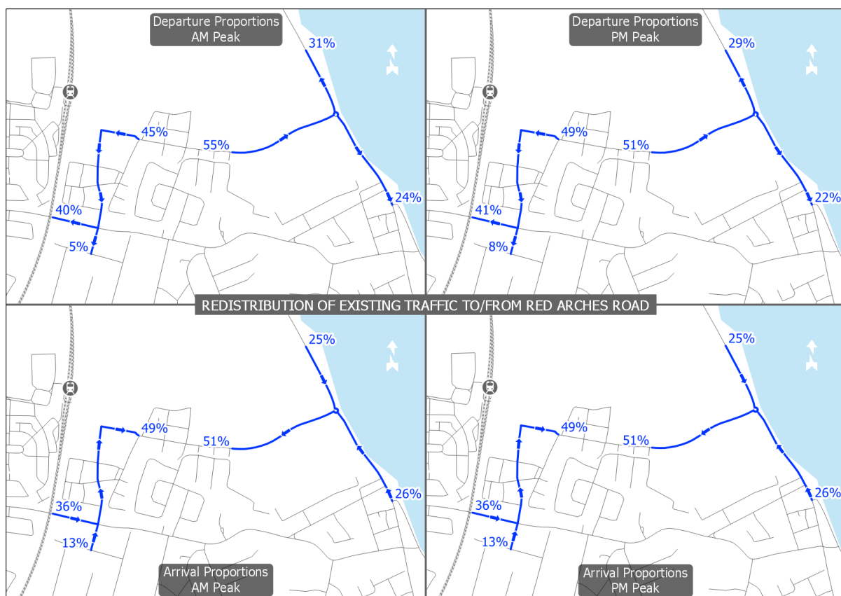
Figure 17.10: Redistribution of Existing Red Arches Road Traffic (Sources: OSi, OSM Contributors)
