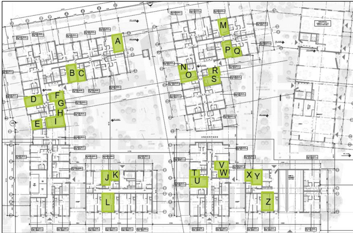
Figure 15.17: Blocks G1/G2/G3 Ground Floor– Average Daylight Factor Assessed Rooms
